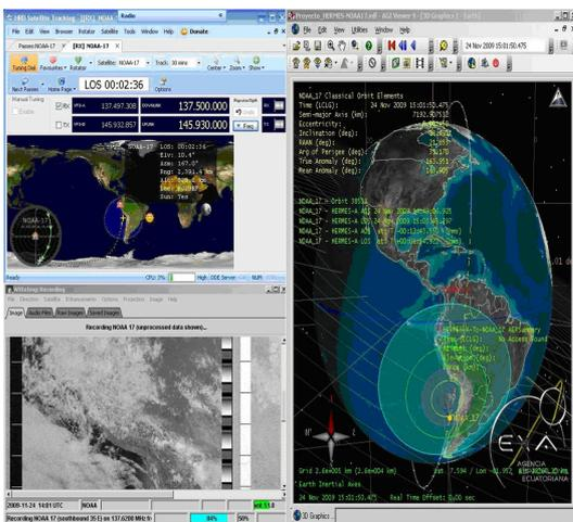
Fig. 11: A real-time STK simulation shows Keplerian elements while capturing NOAA-17 in delta mode operation.
