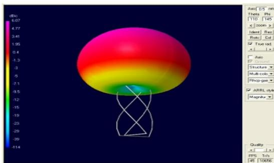
Fig. 6: QHA RHCP radiation pattern. Adapted from <http://homepages.ipact.nl/~pa1are/QHA.html><sup>16</sup>
