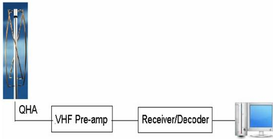
Fig. 2: Typical standalone APT Receiving system
