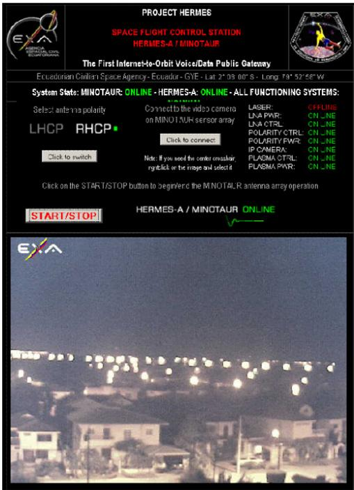
Fig. 10: The communications control using HERMES Web Interface to run/stop, antenna polarity change and onboard IP camera. The most important interface for remote users.
